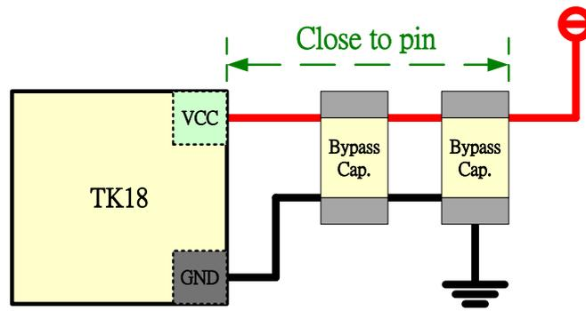
**The trace for internal LDO bypass capacitor:**
