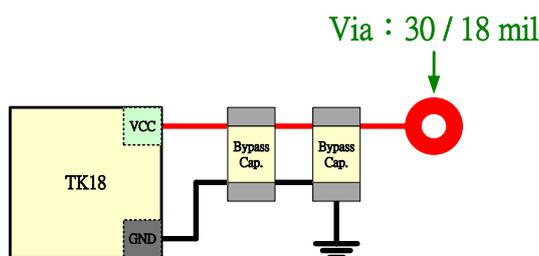
**Note:** The VCC traces between VCC and TK18 should go through the decoupling capacitors instead of routing branches to capacitors. The decoupling capacitors should be placed as close to the TK18 VCC pin.
