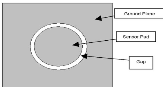
A typical round shape sensor pad is illustrated above. There is a round gap that isolates the sensor pad and the ground plane.
