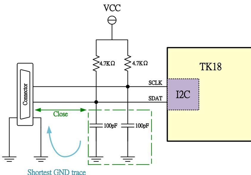
TK18 support I2C bus speed up to 200 KHz.
