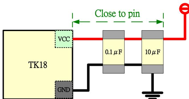
**Note:** For EFT +4KV test, adding a 100uF bypass capacitor to power input is recommended.
